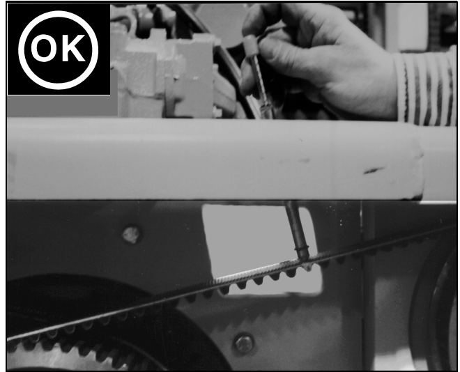
Figure 6 - 27 Tester Used Correctly (side view)
