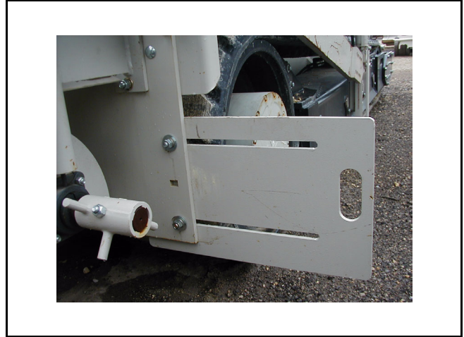
Figure 3 - 45 Material Plate Extended Maneuvering On Hot Asphalt
