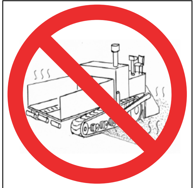
Figure 3 - 48 Do Not Park On Hot Asphalt
