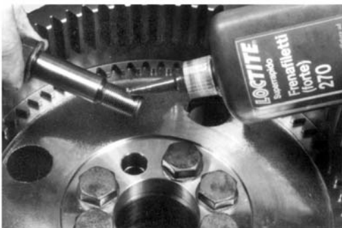
Insert the pilot bolts by using LOCTITE 270 only on the thread.
