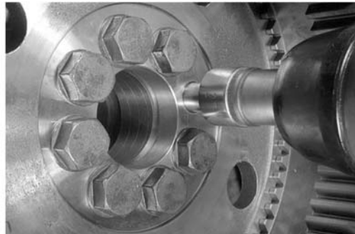
Remove the pilot bolts and mark the crown before disassembly.
