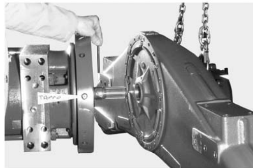
Fix the boogie, and remove it from central body.
