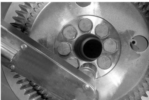
Tighten the pilot bolts with a torque wrench 460-465 Nm.
