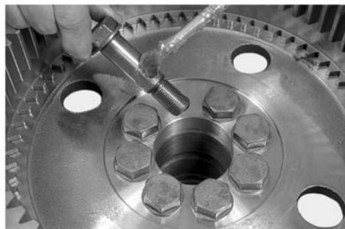
Grease the not threaded part of pilot bolt.
