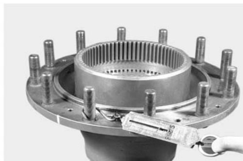
Check the continuous rolling torque on the hub assemble with new bearing and seal ring. Rolling torque from 30 to 40 Nm.
