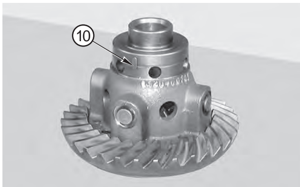
FIGURE 52: ONLY IF PREVIOUSLY DISASSEMBLED Position the key (10) in the differential unit (11).
