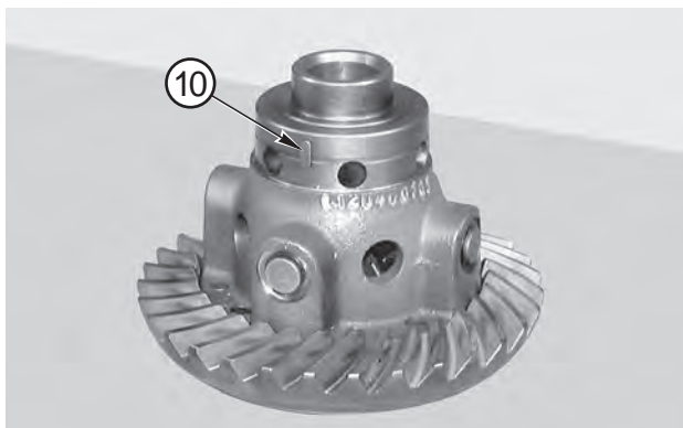
FIGURE 8: ONLY IF NECESSARY Remove the key (10).
