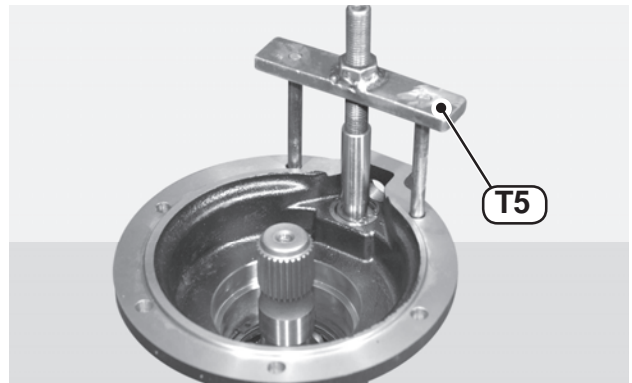
FIGURE 37: Install tool T5 (See drawing T5 p. 63) on the thread of the piston (30) to compress the spring (32) and open the seat for installing the snap ring (34).
