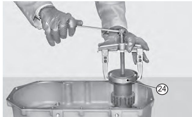
FIGURE 10: Using an extractor, remove non-input side bearing (24).
