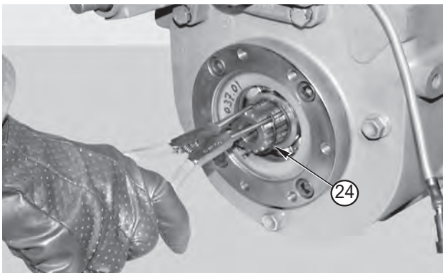
FIGURE 9: Only if reduction gear needs removing: Remove the snap ring (24).
