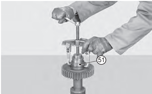
FIGURE 25: Using a puller, remove the bearing (51) inner ring.
