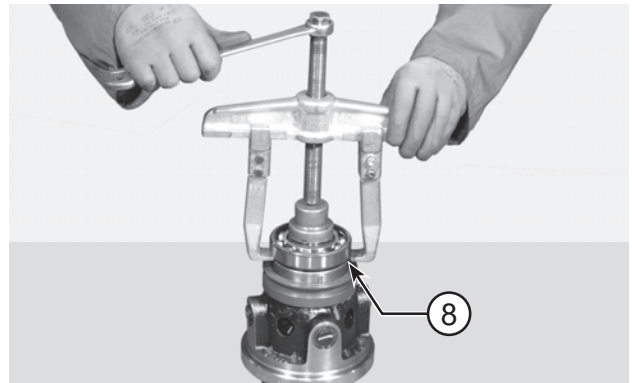
FIGURE 6: Using an extractor, remove the bearing (8).
