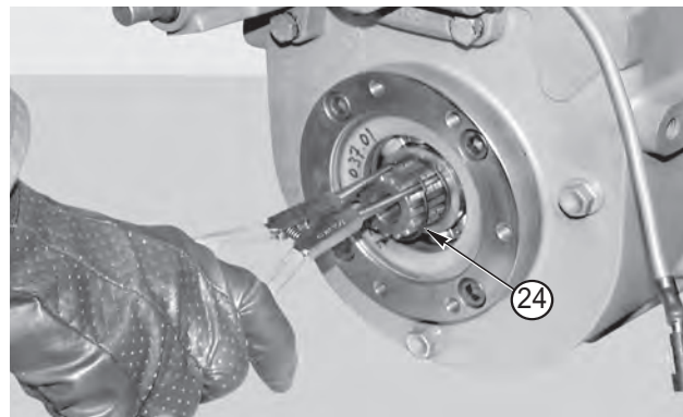
FIGURE 19: Only if previously removed: Install the snap ring (24).
