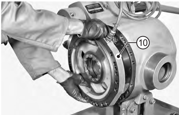
FIGURE 8: Introduce low-pressure compressed air through connection and make sure that the lock control piston comes out at end of stroke. Remove safety studs, rotate cover (10) to an angle of about 45° and remove cover.
