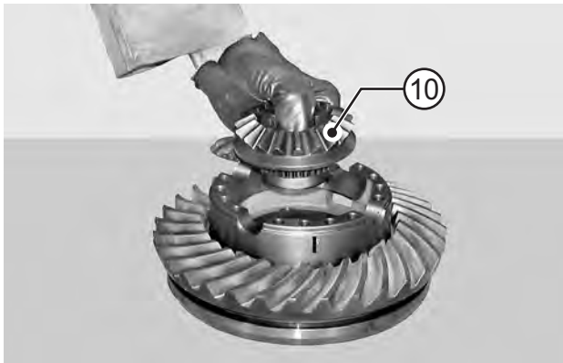
FIGURE 6: Remove the 2nd planetary gear (10).
