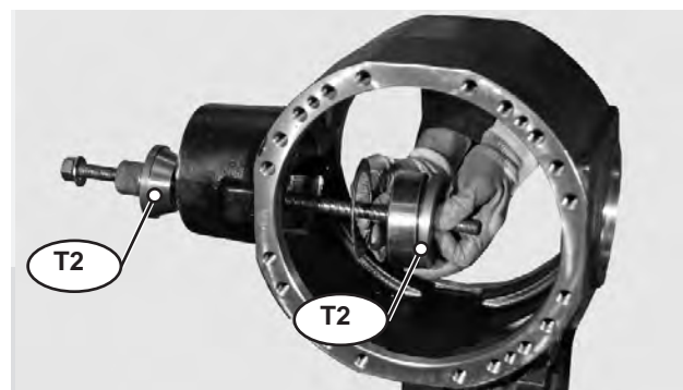
FIGURE 19: Using special tool T2 (See drawing T2 p. 65). Partially insert the bearing cup of the bearing cones (6) and (10) and shims (9).
