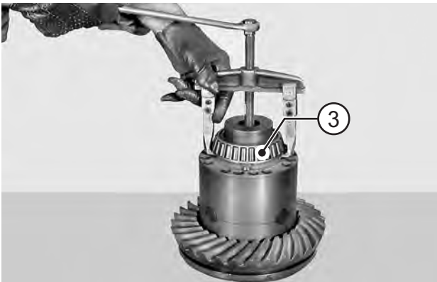
FIGURE 2: Using a puller, remove bearing (3).
