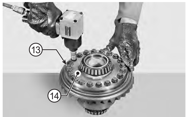
FIGURE 5: Loosen and remove the check screws (13) of ring gear (14).
