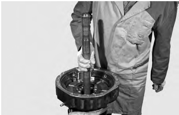
FIGURE 2: Remove the axle shaft.
