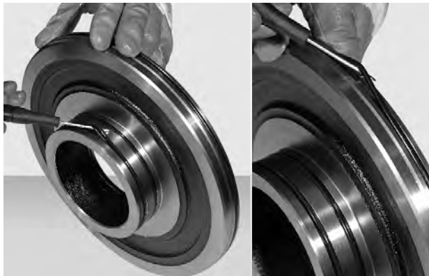
FIGURE 25: Fit o-ring (2) and (4) and anti-extrusion ring (18) onto the piston (3).
