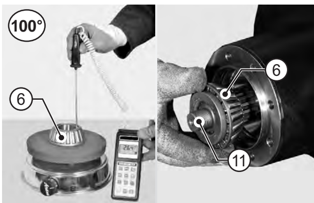
FIGURE 29: Heat the external bearing cone (6) to a temperature of about 212 F° [100 C°] and fit it on to the pinion (11) so as to complete the pack as shown above.
