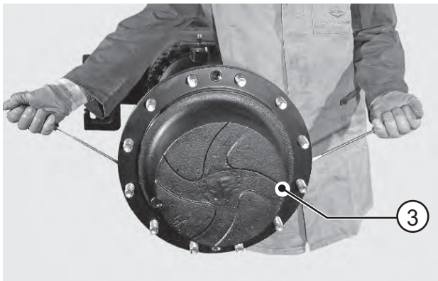
FIGURE 3: Using two screwdrivers or two levers inserted in the slots provided, disjoin the planetary cover (3) away from the wheel hub (16).
