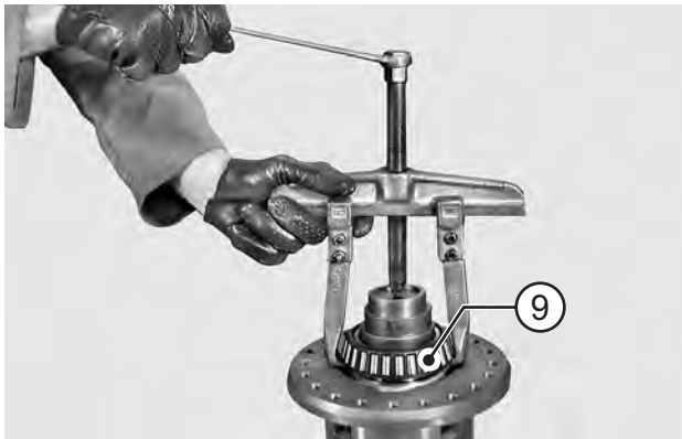
FIGURE 7: Using a puller, remove bearings from ring gear (9) side.
