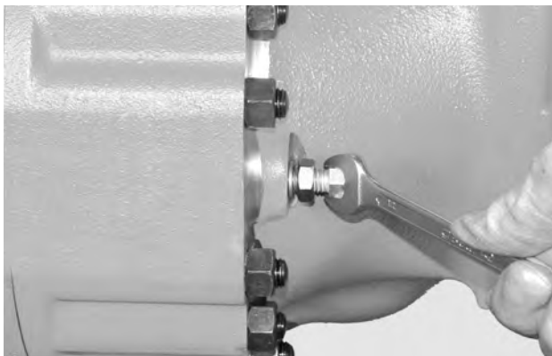
FIGURE 3: Using a wrench, tighten the screws (23) in an alternate sequence by 1/4 turn at a time so as to compress the Belleville washers (1) and disengage the braking disks.
