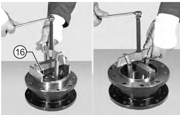
FIGURE 9: With the help of an extractor, remove the thrust blocks (4)(16).
