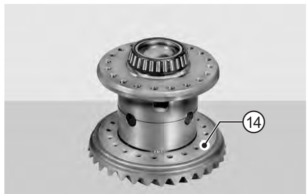
FIGURE 6: Remove the ring gear (14).
