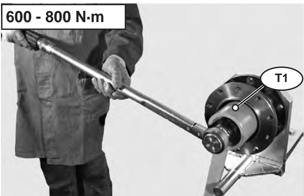
FIGURE 25: Lock the wrench T1 (See drawing T1 p. 77), rotate the pinion using a torque wrench, up to a minimum required torque setting of 600 - 800 N-m.
