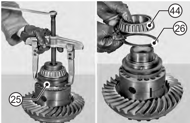
FIGURE 19: DISASSEMBLING THE DIFFERENTIAL GEAR With a puller applied under coupling (25), remove bearing (44) and shoulder shim (26) for coupling (25).
