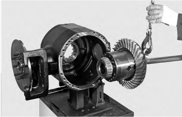
FIGURE 1: Remove the intermediate cover and the whole differential unit. For details, see DIFFERENTIAL UNIT p. 47.
