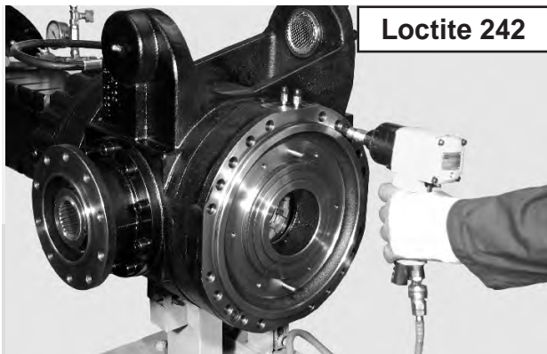
FIGURE 36: Insert the screws (29) and tighten them alternately. Lock the cylinder (17).
