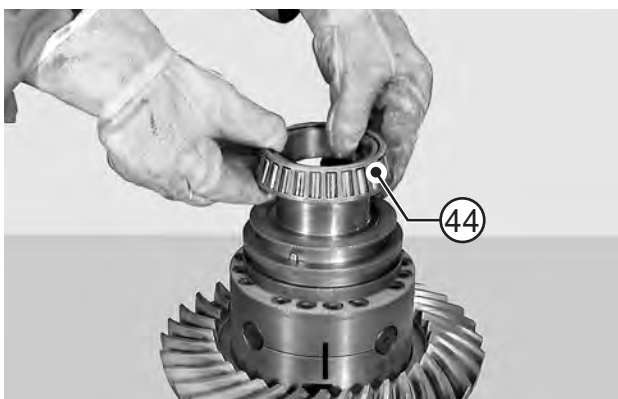
FIGURE 28: Heat bearing (44) to approximately 194 F° [194 F° [90 C°]] and install on the differential.
