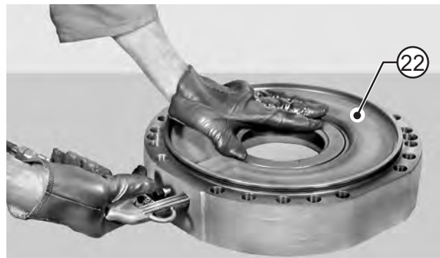
FIGURE 18: DISASSEMBLING THE BRAKE PISTON Gently introduce low-pressure compressed air through the connection of the working brake line and eject the whole piston (22).
