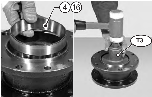
FIGURE 12: Using tool T3 (See drawing T3 p. 78), insert the thrust blocks of bearing (4)(16).
