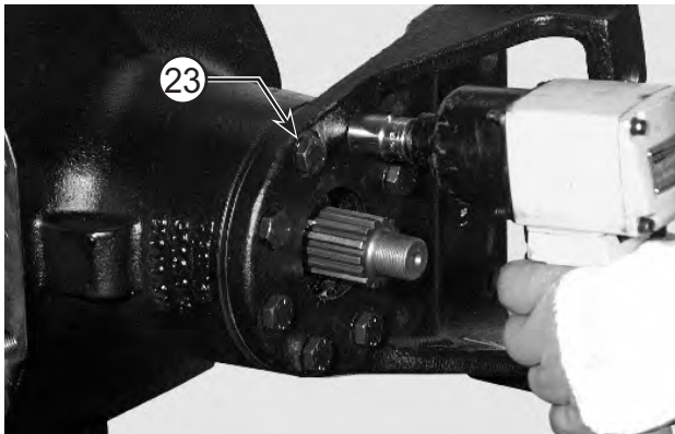
FIGURE 7: Remove the retainer screws (23) and washers (3).
