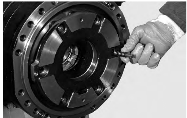
FIGURE 17: Remove the reversal springs (9) and screws (10).
