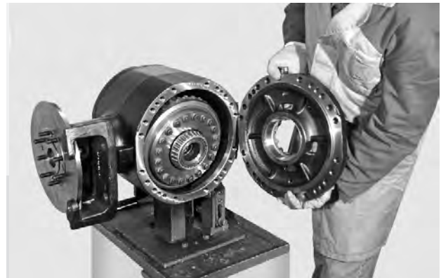
FIGURE 6: Remove the cover and studs.
