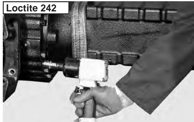
FIGURE 51: Temporarily lock the arm with nuts previously coated with Loctite 242; tighten lightly to make the unit touch the main body.
