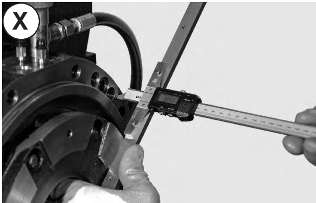
FIGURE 42: Take the measurement from the surface of the intermediate disk to the cover sealing surface with 20 - 35 bar of pressure introduced. EXAMPLE: 30,6 mm
