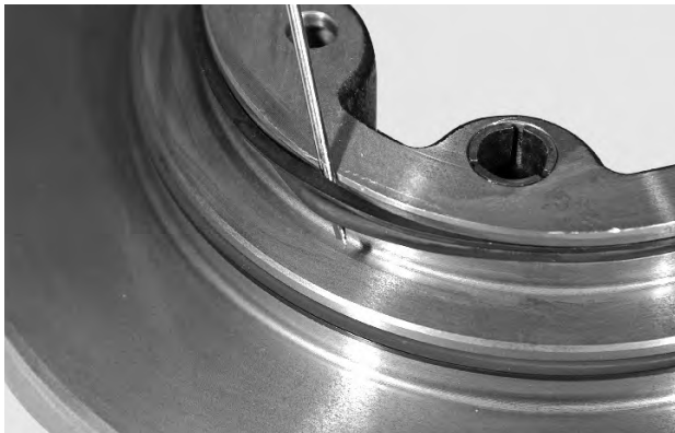
FIGURE 7: Fit o-ring (11)(16) and back-up ring (10)(17) onto the piston (11). Lubricate the piston and the o-rings and install the unit into the arm.
