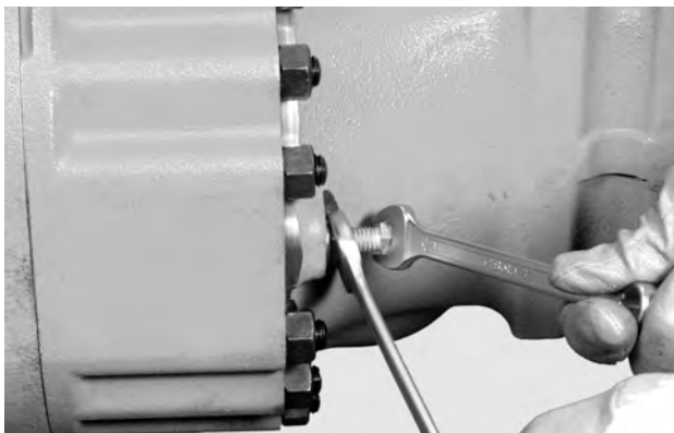
FIGURE 6: Lock into position with nuts (22).
