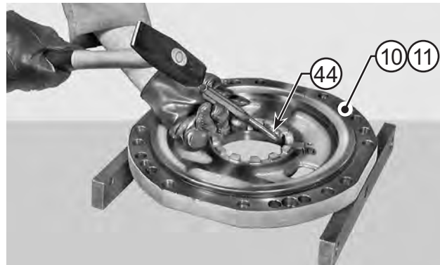
FIGURE 17: If bearings need replacing, remove the outer thrust blocks of bearings (44) from intermediate covers (10) and (11).
