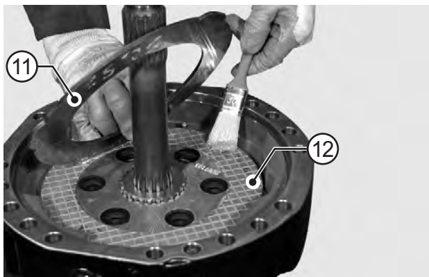
FIGURE 49: Insert the brake discs (11) and (12) in the right sequence.
