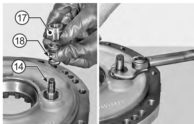
FIGURE 31: Fit spring (18) and ring nut (17) on piston (14). Tighten the ring nut by a few turns, apply a coat of Loctite 242 to the ring nut and tighten to a torque of maximum 50 N·m using a torque wrench.
