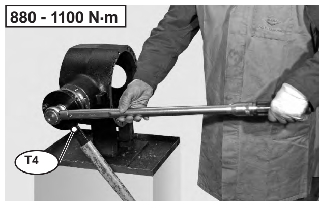
FIGURE 31: Apply torque wrench to the ring nut (1) and special tool T4 (See drawing T4 p. 67) to the pinion (11). Lock the wrench T4 (See drawing T4 p. 67) and rotate the pinion using a dynamometric wrench, up to a minimum required torque setting of 880 - 1100 N·m.
