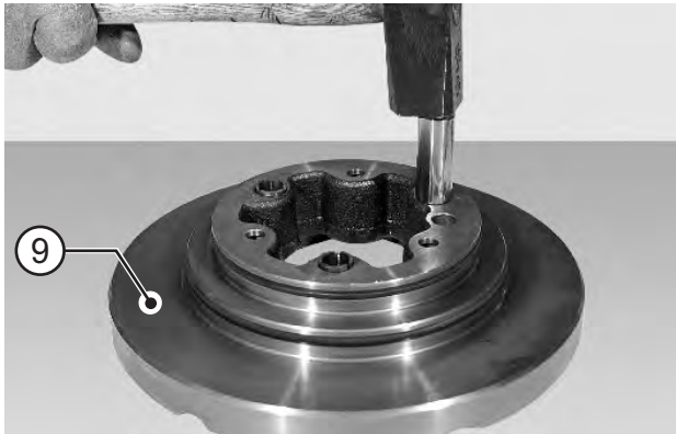
FIGURE 6: Insert the stroke automatic regulation springs (6); place them in line with the piston (9).
