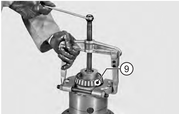
FIGURE 8: Using a separator and a puller, remove bearing from non ring gear side.
