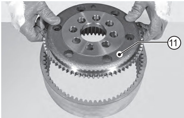
FIGURE 15: Remove the crown flange (11).
