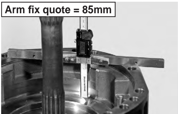
FIGURE 44: Arm fix quote = 85 mm
