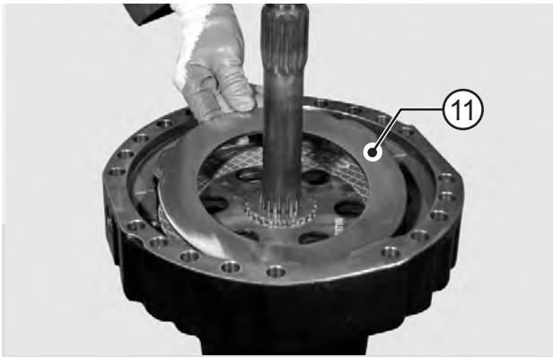
FIGURE 13: Remove braking discs (11)(12), noting down direction of assembly.
