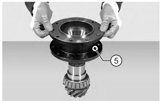
FIGURE 21: Insert the cover (5).
