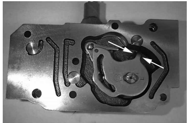
Underside of MDC Module Showing Where to Clamp Locking Pliers
