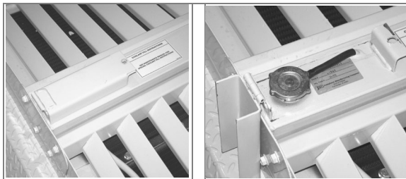
Figure 16. Radiator Fill Location
