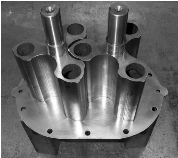
Figure A1. Rotors Assembled on Drive End Plate (Model 4000 with tri-lobe rotors shown)
