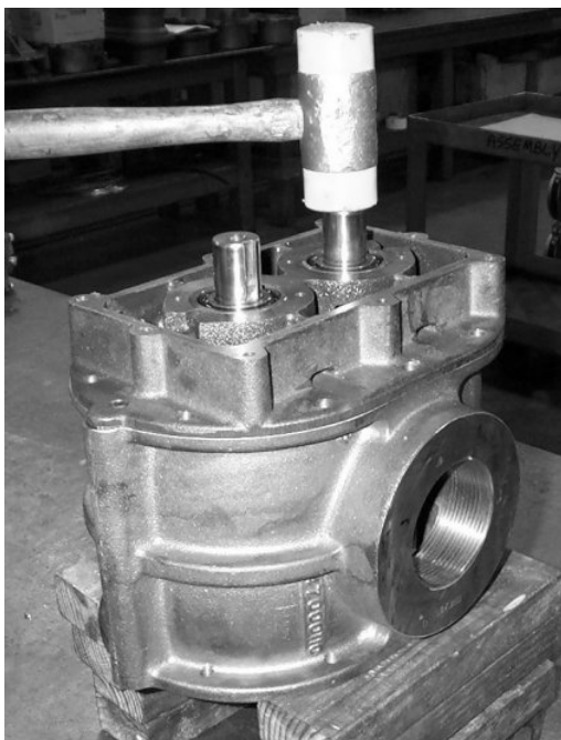
Figure 6. Driving Rotors Out Using Soft
