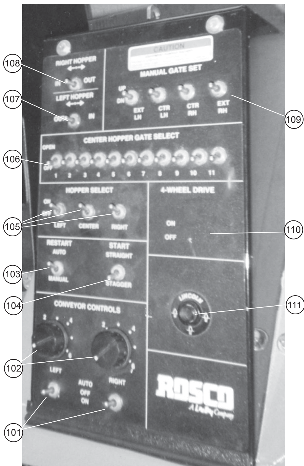
Figure 6 SpreadPro - Right Hand Side Console Controls
