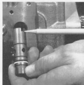
Fig. 83 - Slot in Control Sleeve
