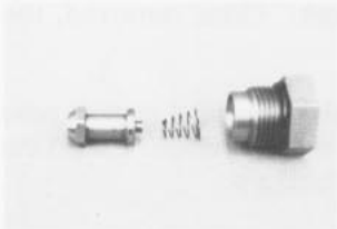
Fig. 35 - Charge Check Valve Components (Through 87-39)
