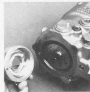
Fig. 47 - Remove Gerotor Cover (Later Units)
