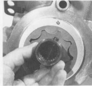
Fig. 66 - Install Drive Coupling (Earlier Units)
