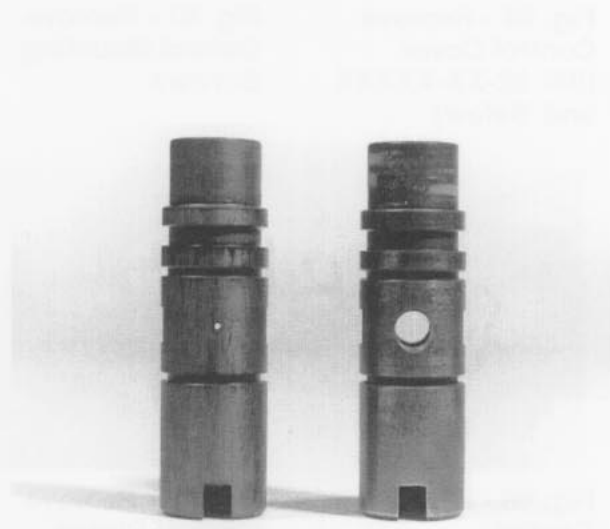
Fig. 82 - Control Valve Sleeve Drain Orifices
