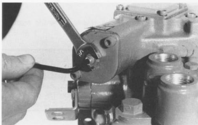
Fig. 25 - Adjusting Neutral for Hydraulic Displacement Control (HDC) or Electric Displacement Control (EDC)
