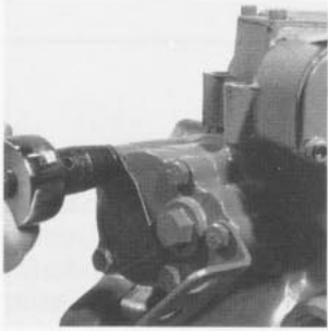
Fig. 15 - Remove Servo Cover (Opposite Neutral Adjustment)
