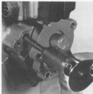
Fig. 18 - Remove Control Orifice (Neutral Adjustment Side)
