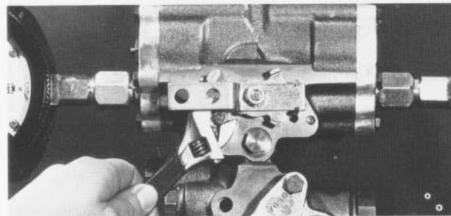
Fig. 23 - Loosen Neutral Bracket Retaining Screw
