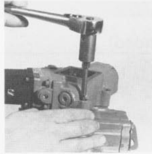
Fig. 87 - Remove Control Mounting Screws
