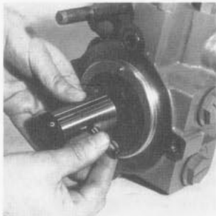
Fig. 59 - Remove Shaft Coupling (Earlier Unit Shown)
