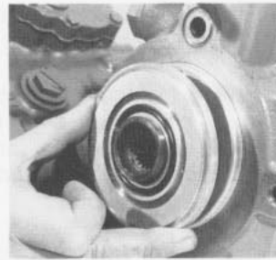
Fig. 68 - Install Gerotor Plate (Earlier Units)
