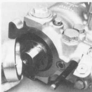
Fig. 61 - Remove Gerotor Cover (Later Unit)
