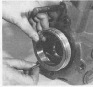
Fig. 64 - Orienting Gerotor Ring and Pin (CCW) (Earlier Units)
