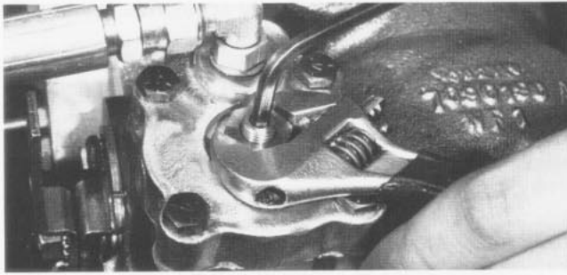
Fig. 20 - Loosen Neutral Adjustment Lock Nut
