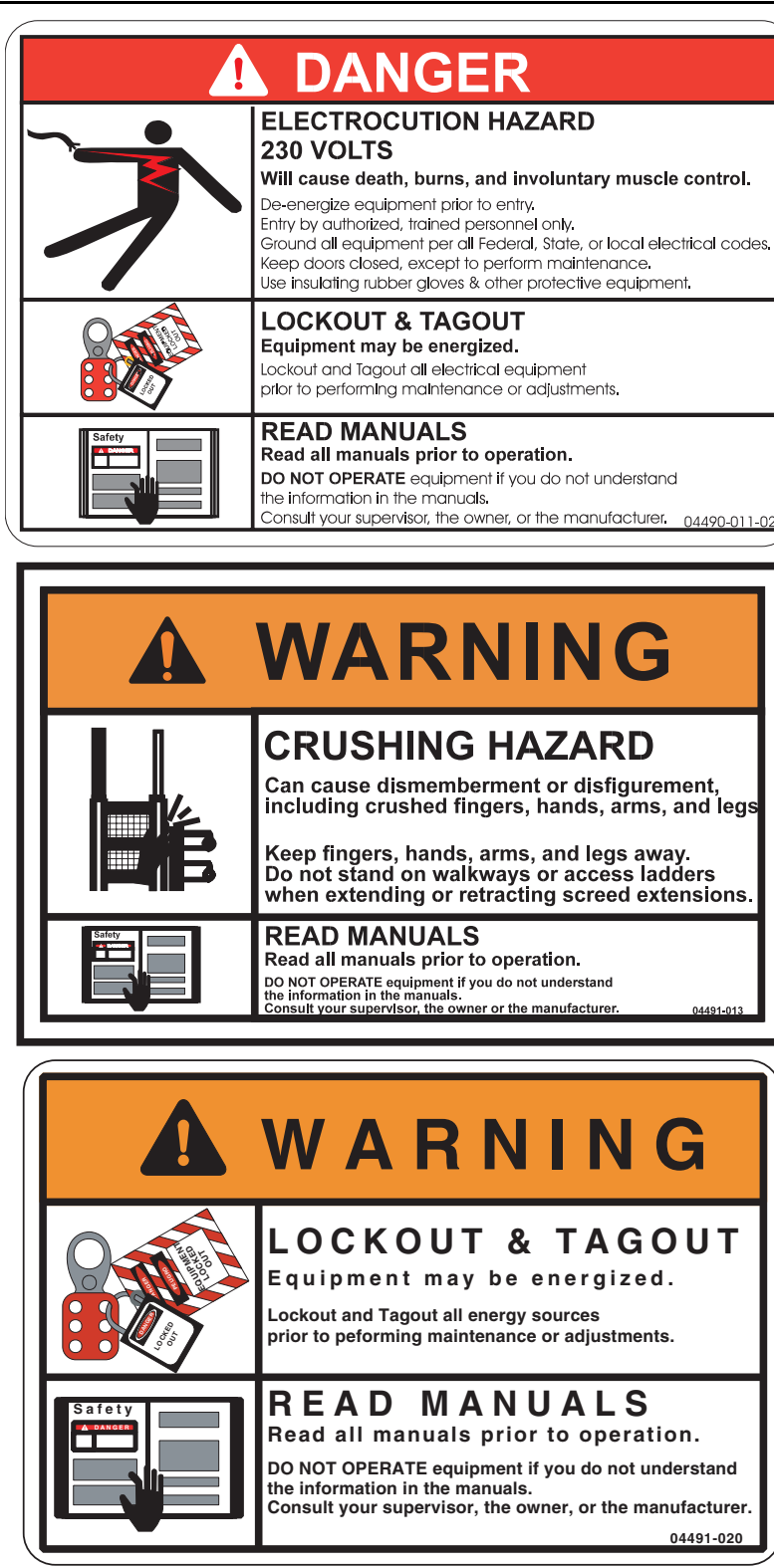
Figure 2 - 6 Screed Danger and Warning Decals
