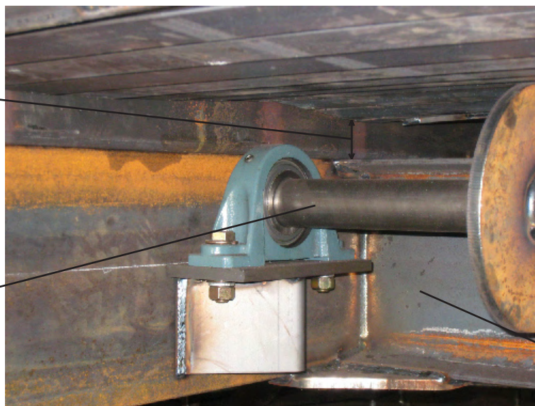
Adjusting screw for the infeed conveyor chain tension
