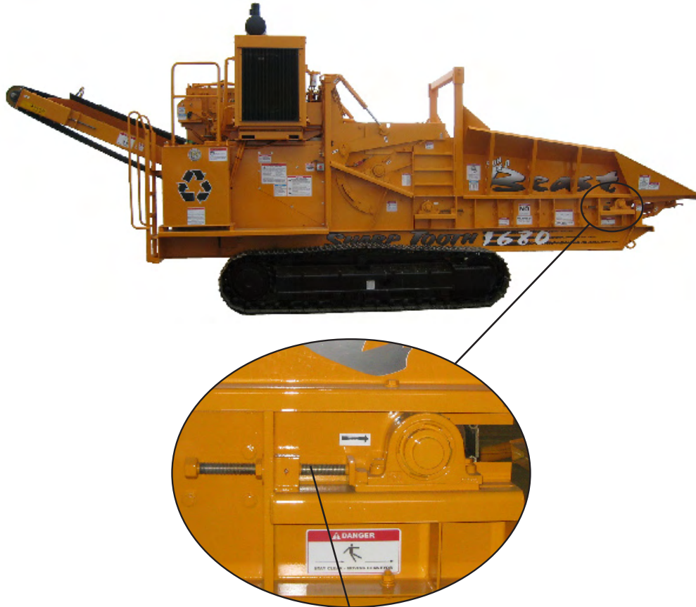
Adjusting screw for the infeed conveyor chain tension
