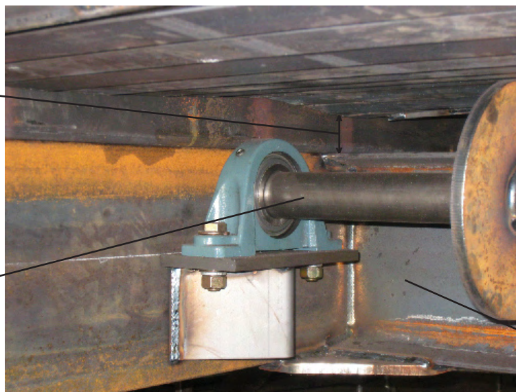
Adjusting screw for the infeed conveyor chain tension
