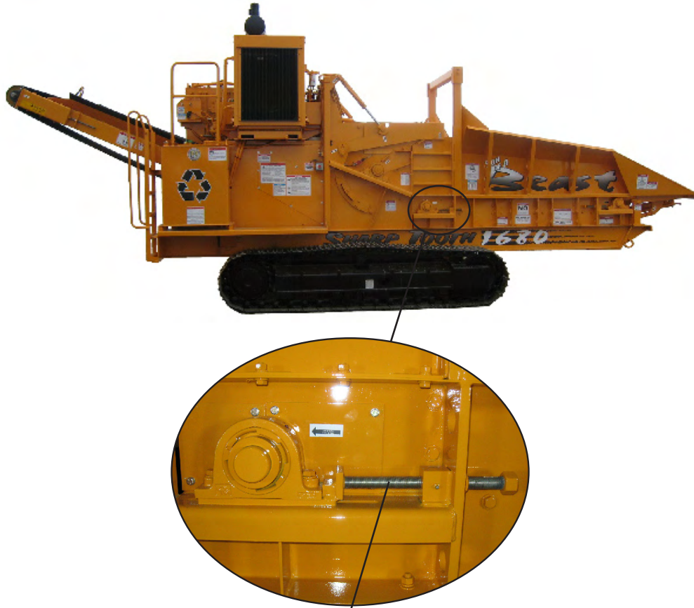
Adjusting screw for infeed conveyor to anvil clearance
