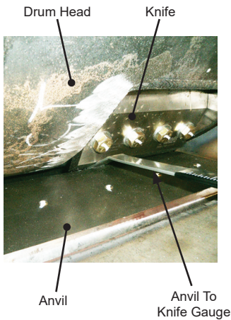
View looking through the feedwheels at the throat area
