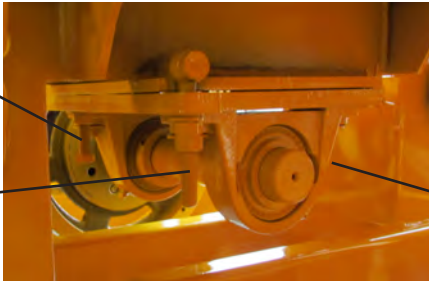
Jack Shaft Bearing
