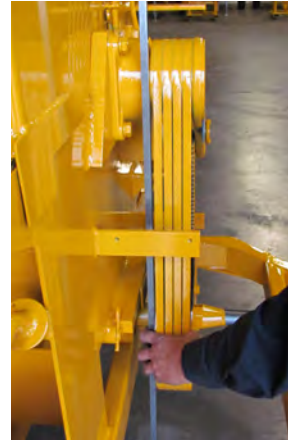
Check sheave alignment with straight edge.
