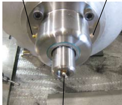
Grease zerk on end of stub shaft
