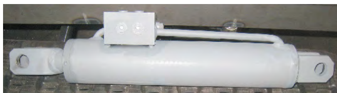
Swing Cylinder: 900-3958-81 Counter Balance Relief: 900-3944-87
