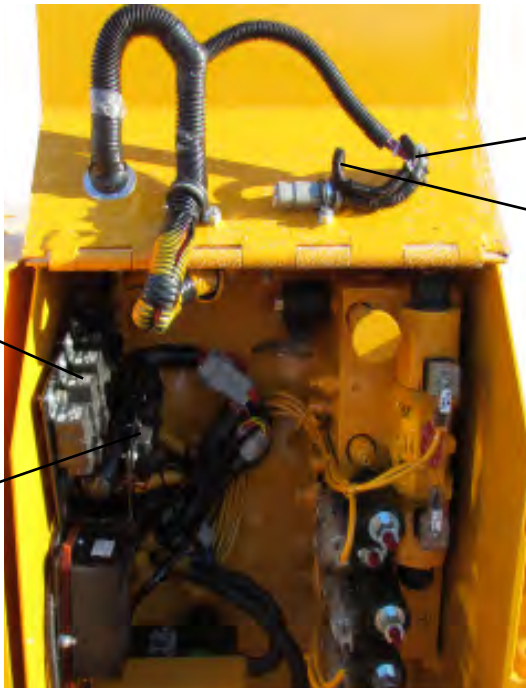
MACHINE HARNESS - DIESEL ENGINE & REMOTE CONTROLS (992-8000-20) Relay Harness w/ Bracket & Hardware (992-8000-18) 12 Volt Fused Relay Harness (204-8000-02)
