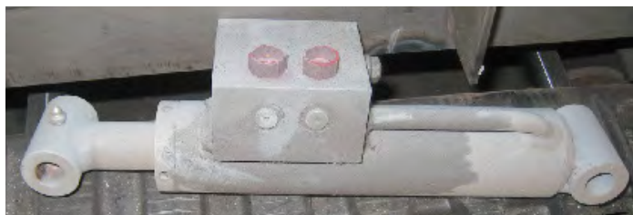
Scrape Blade Cylinder: 900-3941-35 Counter Balance Relief: 900-3944-87
