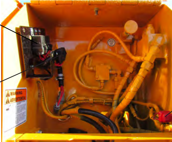
MACHINE HARNESS - DIESEL ENGINE & SWING OUT CONTROLS (204-8000-07) Relay Harness w/ Bracket & Hardware (992-8000-16) 12 Volt Fused Relay Harness (992-8000-13)
