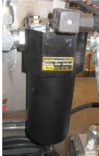
CUTTER PUMP CHARGE FILTER
