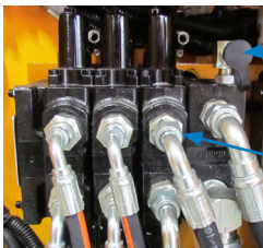
Pressure Gauge Port (Left Track, Track Extend, Cutter Up/Down)
