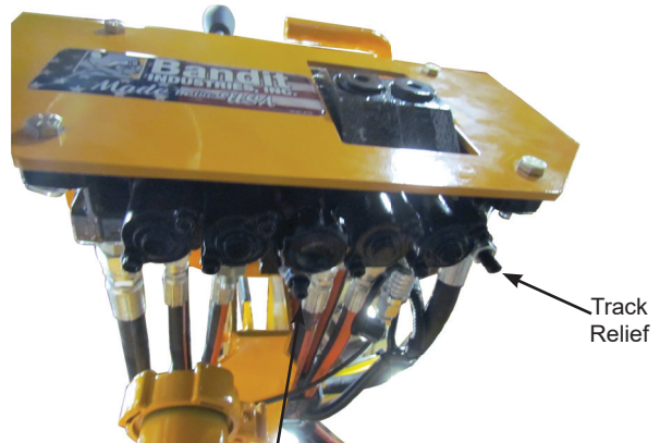
Cutter Head Swing Left/Right & Cutter Head Up/Down Relief
