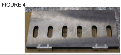
IMPROPER USE OF BABBITT ON CHIPPER KNIVES
