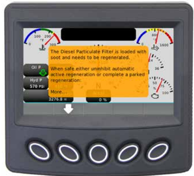
Figure 4-22. Regen Caution Message Popup Screen Example Requiring Use of UP/DOWN Soft Keys
