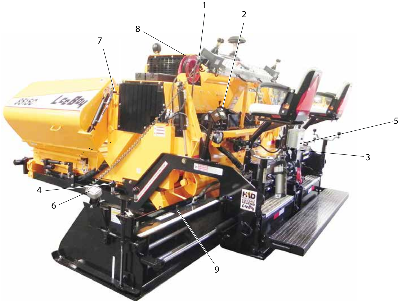
Figure 3-8. Left Side Controls
