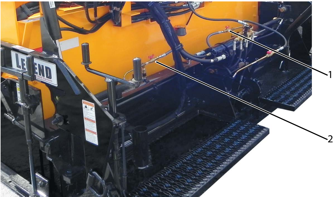
Figure 3-8. Extension Burner Controls
