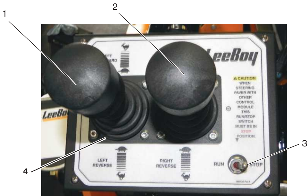
Figure 3-3. Steering and Speed Control Box
