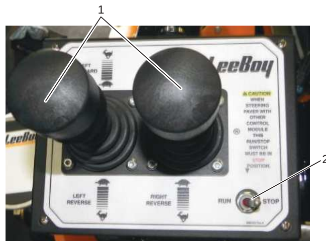
Figure 4-30. Steering and Speed Control Box
