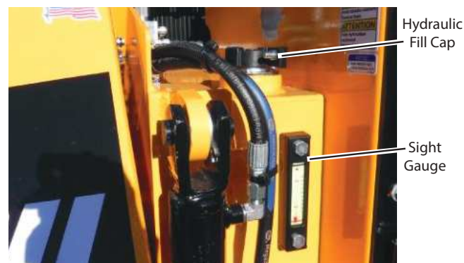
Figure 5-18. Hydraulic Oil Cap and Sight Gauge
