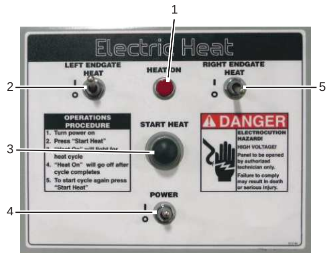
Figure 4-58. Electric Heat Controls with Endgate Switches
