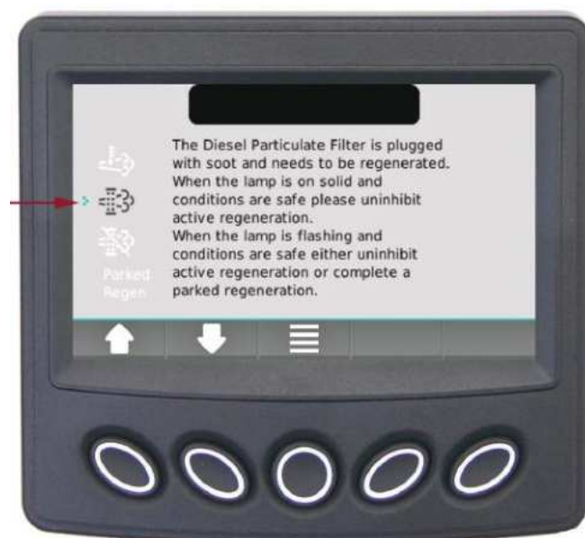
Figure 4-12. Needs Regenerating Screen
