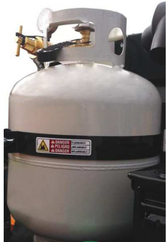
Figure 3-9. Propane Tank Controls
