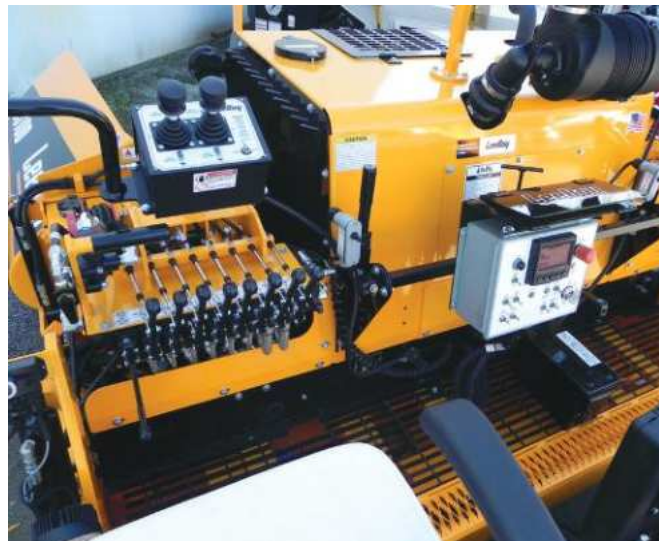
Figure 4-29. Operator Control Station
