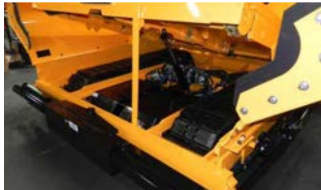
Figure 5-4. Safety Prop in Position
