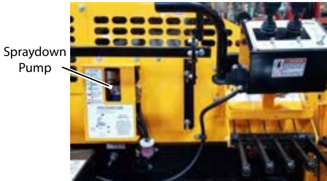
Figure 5-50. Spraydown Pump Location
