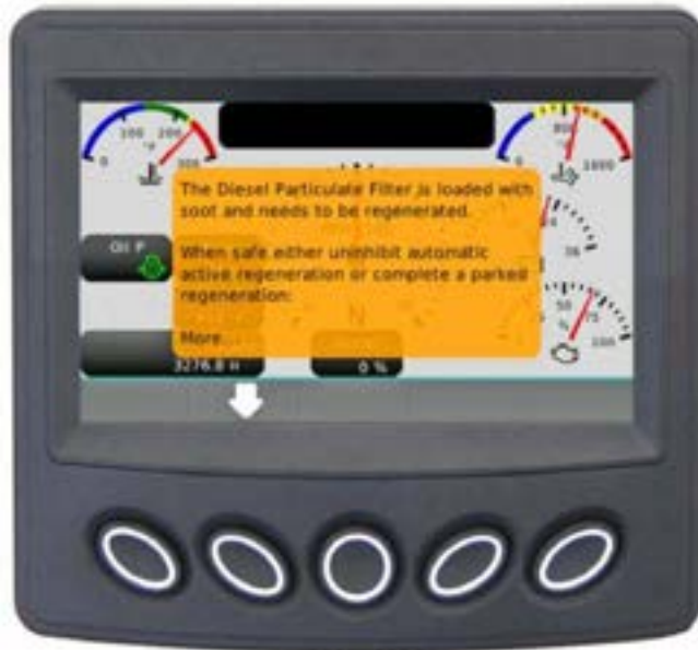
Figure 4-23. Regen Caution Message Popup Screen Example Requiring Use of UP/DOWN Soft Keys
