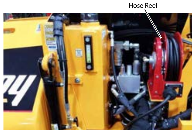
Figure 4-33. Spray Down Hose Reel
