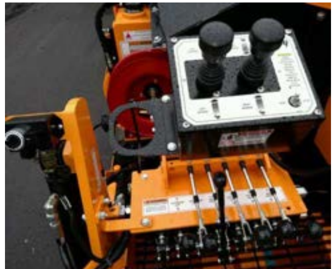
Figure 4-31. Operator Control Station
