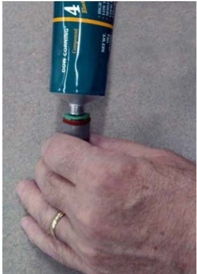
Figure 5-27. Correct Application of Dielectric Grease
