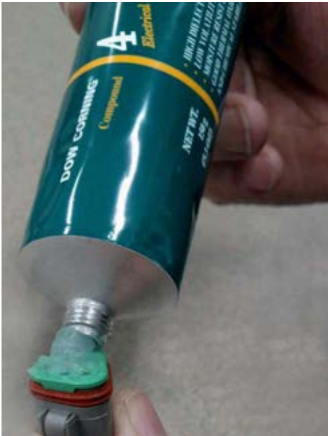
Figure 5-28. Incorrect Application of Dielectric Grease
