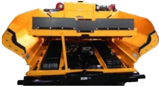
Figure 5-1. Hydraulic Conveyor Bed
