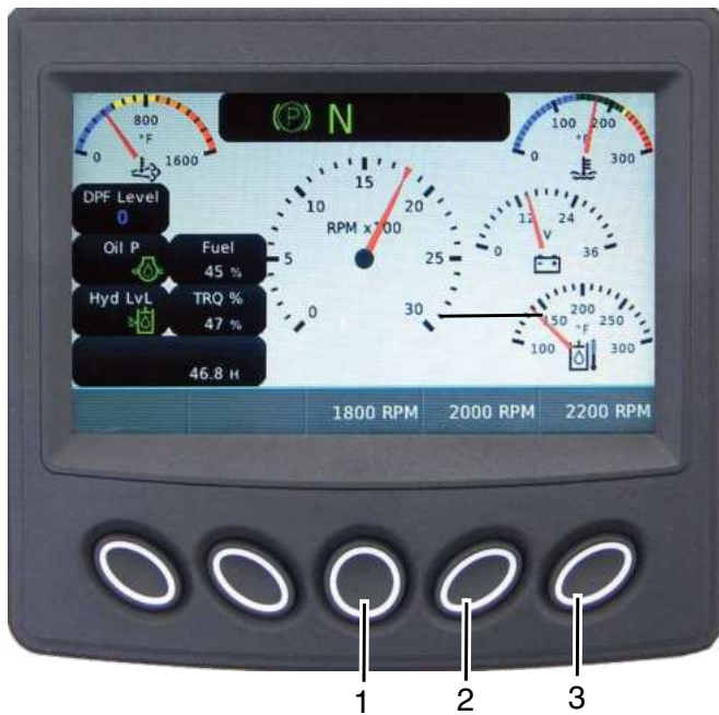
Figure 4-5. Engine Throttle Speeds Screen with Generator ON
