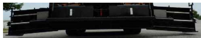
Figure 4-68. Screed Sloping Extensions
