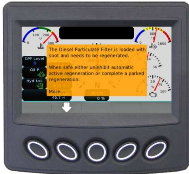
Figure 4-23. Regen Caution Message Popup Screen Example Requiring Use of UP/DOWN Soft Keys
