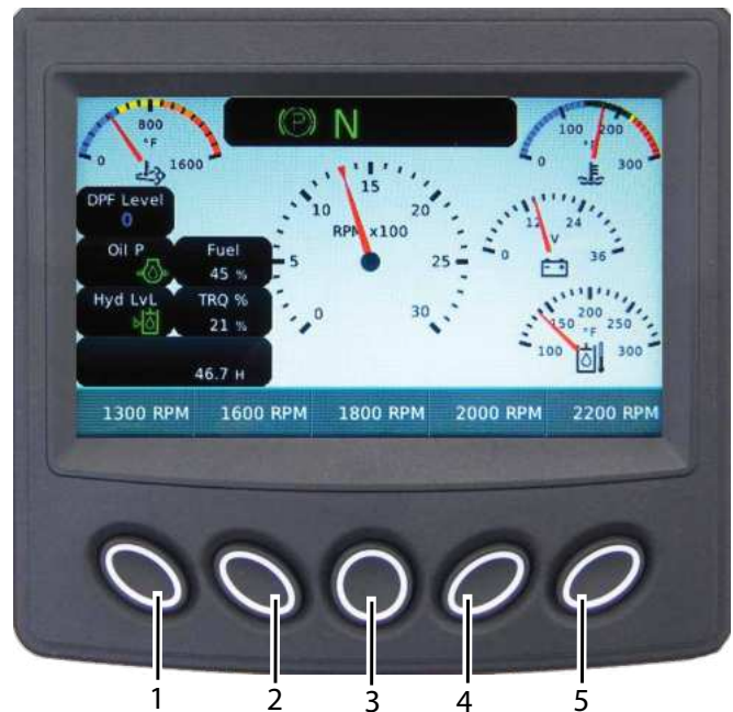
Figure 4-4. Engine Throttle Speeds Screen with Generator OFF
