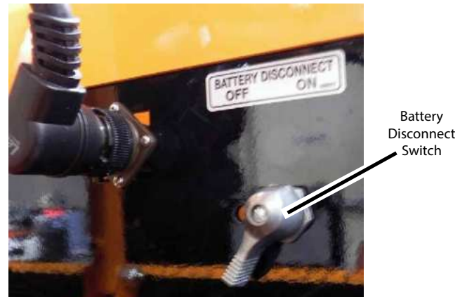
Figure 5-22. Battery Master Switch
