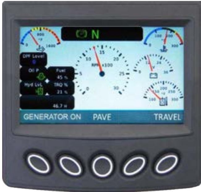
Figure 4-6. Engine Throttle Speeds Screen with Generator ON
