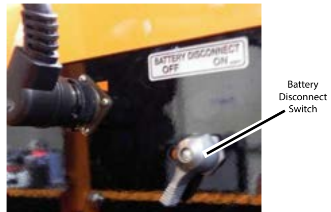
Figure 5-22. Battery Master Switch
