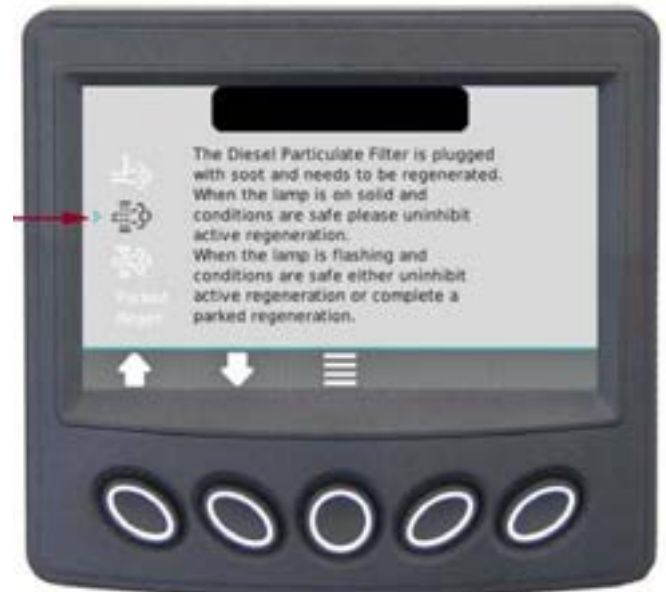
Figure 4-14. Needs Regenerating Screen
