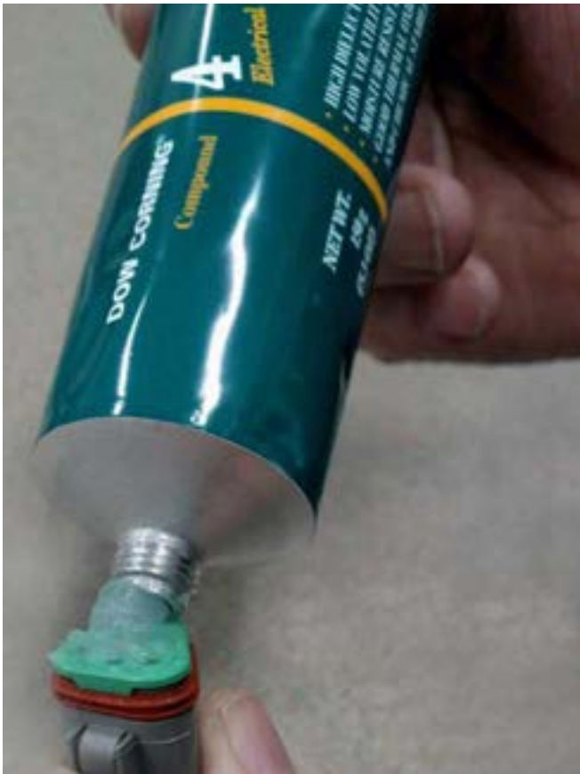
Figure 5-28. Incorrect Application of Dielectric Grease
