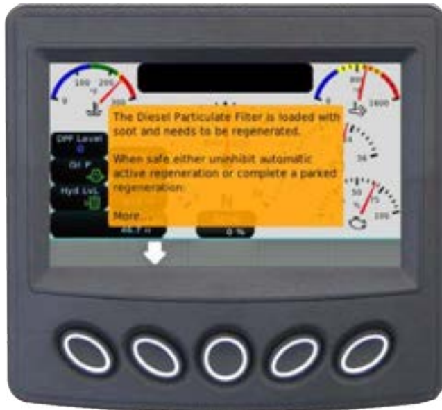
Figure 4-24. Regen Caution Message Popup Screen Example Requiring Use of UP/DOWN Soft Keys
