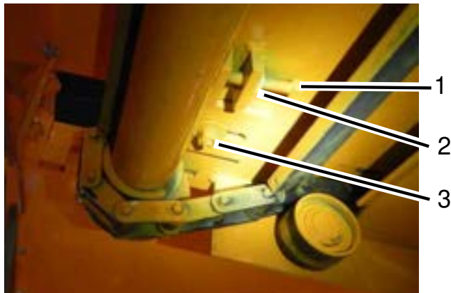
Figure 5-6. Conveyor Flight Chain Adjustment
